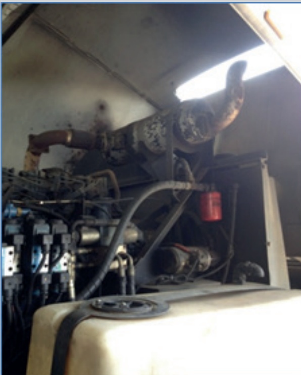
Figure 4: Partial Diesel Particulate Filters fitted to a Blacktown City Council street sweeper; main and stationary engine. Photo: John Bannister, Blacktown City Council
