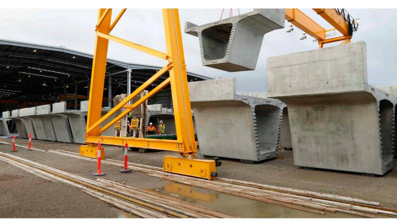
Diesel powered gantry crane in action lifting a 26-tonne concrete segment.
